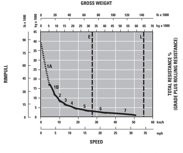
1A – 1st Gear (Converter Drive)
