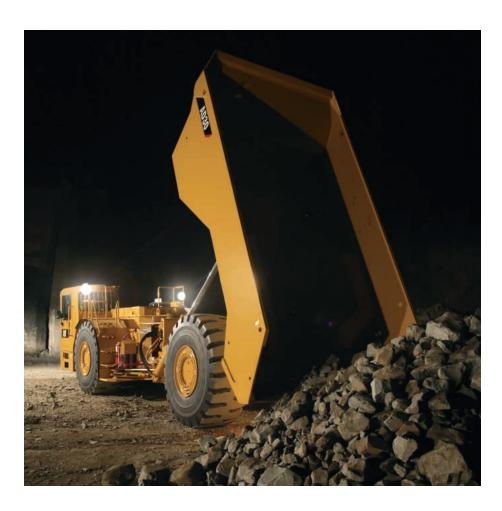
**Truck Payload Management System** (**TPMS**). The optional TPMS system calculates the payload the truck is carrying and determines truck cycle times.
