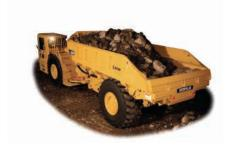
**Ejector Body.** The ejector body offers clean load ejection and the capability to work in areas with restricted overhead clearance and soft underfoot conditions.
