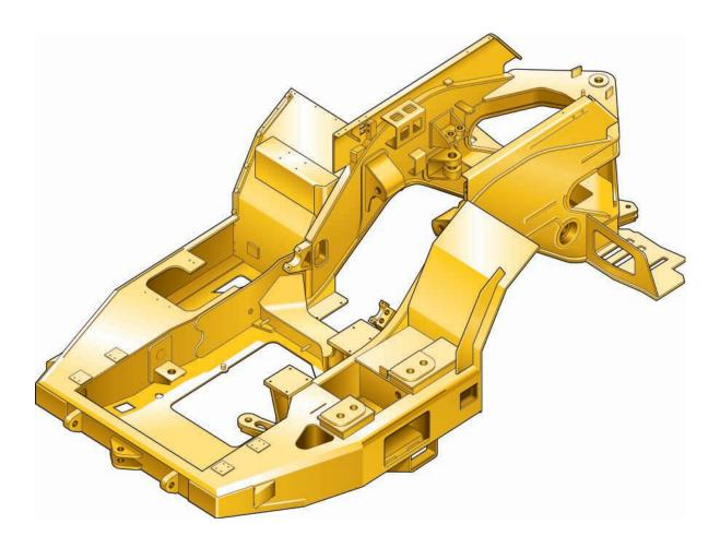
**Frame Design.** The frame incorporates a box-section design with wide and stiff frame beams to handle torque loads. The frame design decreases stress in the hitch area and optimizes suspension geometry. Materials and weld joints are matched to optimize the life of the structure.
