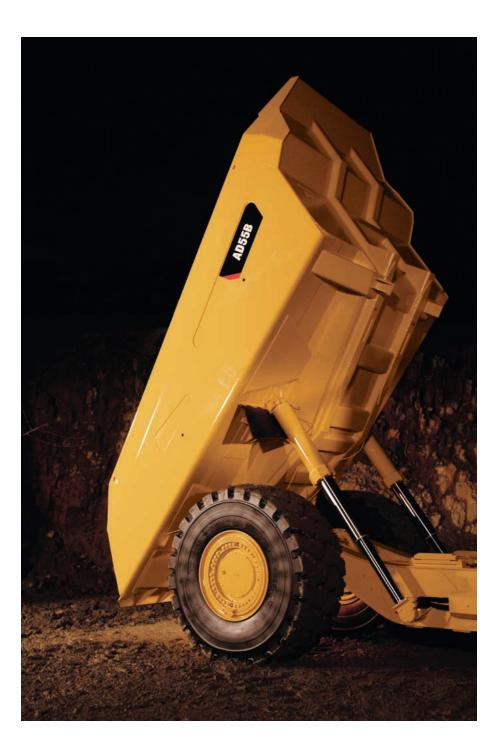
**Ejector Body.** The ejector body offers clean load ejection and the capability to work in areas with restricted overhead clearance and soft underfoot conditions.
