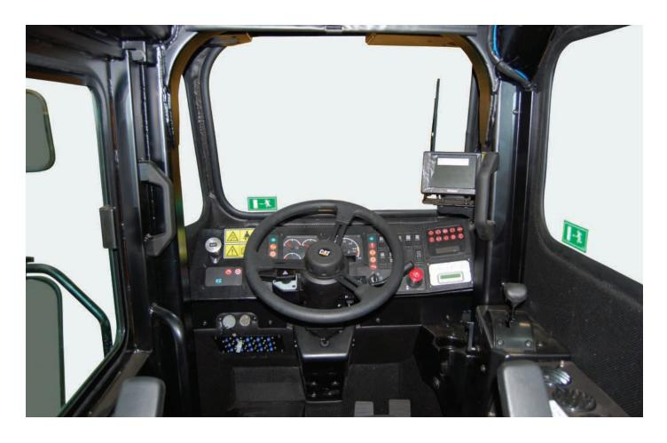
**Ergonomic Layout.** The AD55B operator station is ergonomically designed for total machine control in a comfortable, productive and safe environment. All controls, levers switches and gauges are positioned to maximize productivity and minimize operator fatigue.
