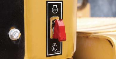
Your Cat G Series truck is designed to provide operators and technicians with easy access to common service points like engine lockout, machine system lockout, fluid level sight gauges, grease fittings and access to the engine for regularly scheduled maintenance.
