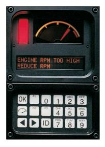
**Keypad.** Provides operator or service technician immediate access to current machine information, gauge values, and stored data through the message center display.
