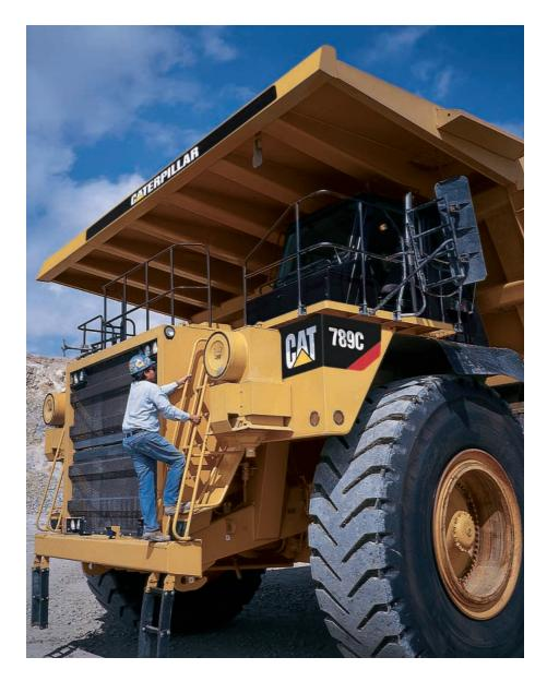
**Overload Policy.** Safety is integral to maintaining the highest productivity in mining machine operation. Caterpillar's 10/10/20 Overload Policy assures that steering and braking systems have sufficient capacity to perform, even at 20% overload.
