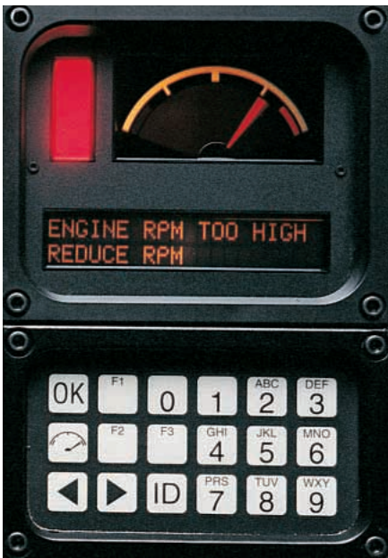
Message Center. Displays messages requested by operator and advises operator of abnormal machine conditions.
