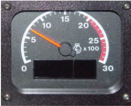
Speedometer/Tachometer Module. Monitors three systems: engine speed, ground speed and actual gear.
