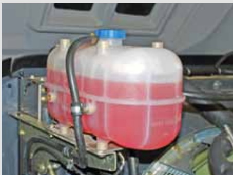
See-through fluid reservoirs and sight gauges let you check fluid levels at a glance.
