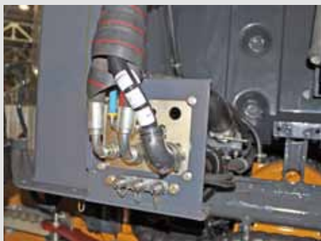
Easily accessible test ports allow technicians to troubleshoot problems more quickly.
