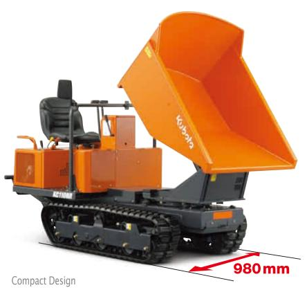
Working in space-restricted environments is easy with the compact KC110HR. The narrow, 980 mm machine width lets it fit into small workspaces, while the compact-but-powerful dumping carrier can rotate tightly with minimal overhang.
