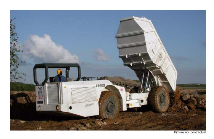
Tunnel articulated Dump Truck PAUS model ITC 10500 with all wheel drive and reverse seat
