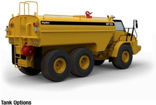
Remote controlled turret monitor, tank bulkhead mounted, hydraulically operated.
