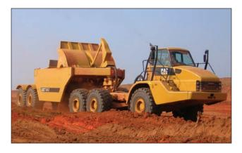
The 7460 Ejector Trailer unloads quickly, due in part to the 1281 mm (78 in) apron opening. The positive bulldozer ejector extends 102 mm (4 in) beyond the front edge of the trailer floor to minimize carryback.
