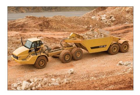
The E-Ject<sup>™</sup> Systems 7460 Ejector Trailer expands the capacity of the Cat<sup>®</sup> 740 Articulated Truck by 40% — move more dirt faster with fewer operators and machines.
