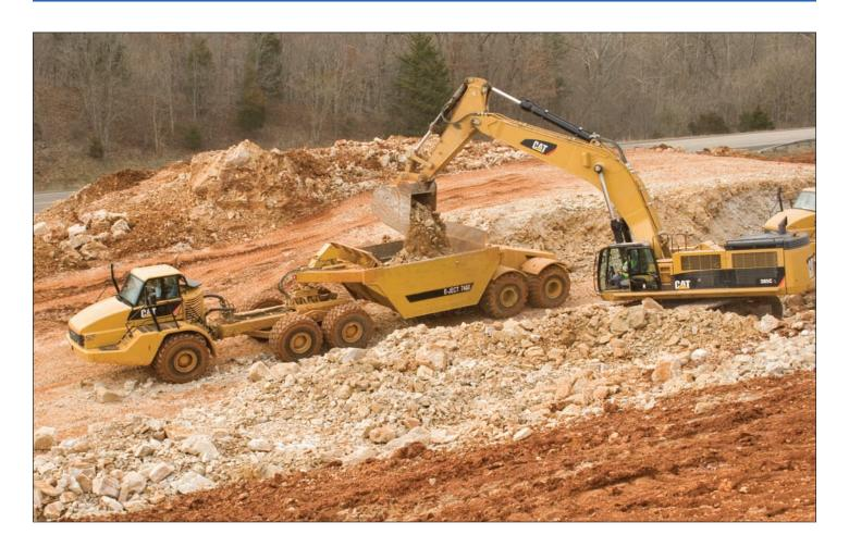
Higher Capacity. With 40% higher capacity than a standard Cat® 740 Articulated Truck, the E-Ject™ 7460 Ejector Trailer provides increased productivity at lower costs. The trailer, which connects to a fifthwheel style hitch installed in place of the truck body, is pulled by rugged and powerful Cat 740 Articulated Trucks.
