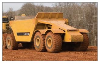
The innovative walking-beam axles allow the tires to oscillate, providing outstanding operator comfort and less haul road pumping.
