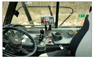
The 7460 EjectorTrailer is easy to operate. A dual-mode (Manual and Automatic), in-cab controller is used to control the trailer's apron and ejector functions.
