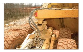
The 7460 Ejector Trailer connects to Cat 740 Articulated Trucks using a 89 mm (3.5 in) diameter pin in a fifth-wheel style hitch installed in place of the truck body and hoist mechanisms. The hitch position is centered between the truck's rear axles for optimal weight distribution when loaded.
