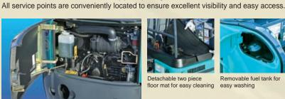
**Engine compartment layout optimised for serviceability**
