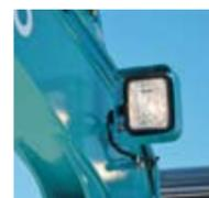
Work lights have been added on both sides to provide a clear view during nighttime operations.
