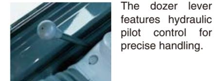
The dozer lever features hydraulic pilot control for precise handling.
