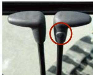
The travel lever is fitted with a button for easy switching to Hi-Mode travel.
