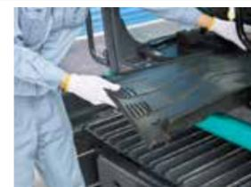
■ Internal and external air conditioner filters can be easily removed without tools for cleaning.
