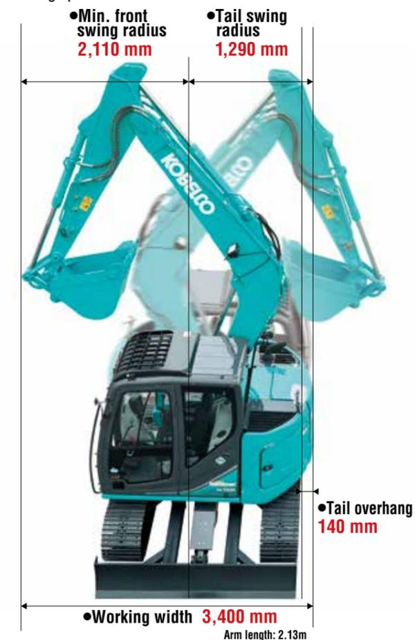
Working width equals the sum of the minimum front swing radius and tail swing radius.
