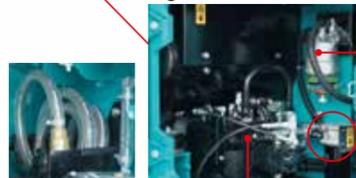
Large fuel filter (with built-in waterseparator)
