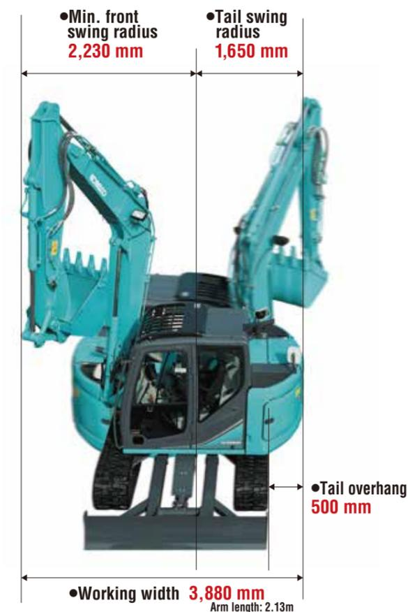
Working width equals the sum of the minimum front swing radius and tail swing radius.
