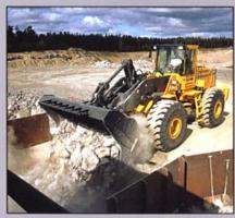
The L180's countershaft transmission is, as with other Volvo BM transmissions, equipped with Automatic Power Shift (APS). Gear changes are made electrically and the operator only needs to choose forward/reverse and kickdown. It's easier than driving a car.
