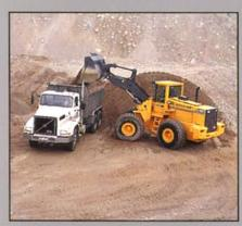
The adjustable boom and bucket kickout mechanism automatically assumes the right position for a level bucket and the optimum height for dumping. High and controlled dumping speeds give short cycle times.
