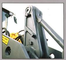
To facilitate regular maintenance, all lubrication and control points are positioned for easy access from ground level. Double-sealed bearings increase dependability and operating life.
