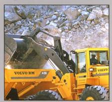
The new loader unit, TP-linkage (Torque Parallel Linkage), is designed for truly demanding construction work. TP-linkage combines the best from Volvo BM's parallel-system with advantages of the traditional Z-linkage.
