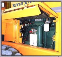
The L180 has a fuel injected, 12 litre, 211 kW (289 hp) Volvo turbo diesel engine with a maximum torque at 1100 rpm. This means low fuel consumption and power to spare to run the hydraulics, for example, when you're backing up with a full load.
