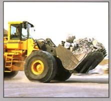
The L180's standard bucket is 4.2 m<sup>3</sup>. It is specially adapted for the carrying position and is held in place against the mechanical stops by substantial hydraulic forces. This ensures good stability and a minimum of spill during load and carry work.
