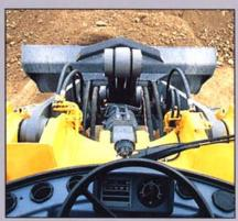
Large windshield and the loader unit's "clean" design gives you good visibility over the wheels and bucket corners. The unique wrap-around windshield ensures a panoramic view, and the easily adjustable rear view mirrors are placed high so as not to block forward visibility.
