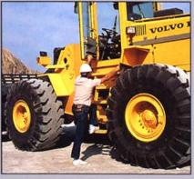
A wide door which opens wide, slipfree ladder with 15 degree tilt and handles which are reachable from ground level make entering the cab easy. Well-placed ladders and handles facilitate inspections and maintenance.
