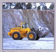
The L180 has new axles of Volvo BM design. The drive axles are fully floating and the front axle has a 100% differential lock. The brake system has dual-circuit, circulation cooled, sealed wet disc brakes for longer life and safety.
