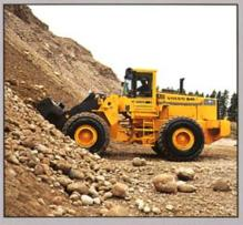
Its unique geometry gives TP-linkage both high breakout torque and parallel action. Thanks to the newly designed T-link, 85% of the breakout torque remains within the whole lifting range. This means you get more breakout power both in the forward and backward tilting positions.
