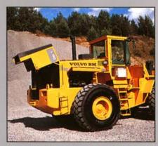
The large radiator hood swings up easily. The radiator is suspended on shock-absorbing hinges and swings out for easy cleaning. The L180 has large, gas-strutted engine covers which fold up as a single unit to facilitate service and inspection.
