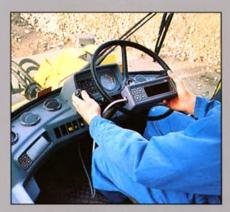
The electronic Contronic monitoring system provides continuous readouts on the loader's condition. Contronic also serves as a handy diagnostic instrument for service personnel for faster servicing and greater availability.
