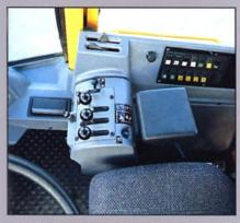
The hydraulics are finger-tip controlled with ease. Controls for forward/back (optional), kickdown and engine braking are also found on the console. This means you can operate all functions with your right hand and steer with your left.
