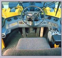
All the information you need on the loader can be found on the new instrument panel. Here's space for the Contronic cab display (optional) which provides continuous readouts on the loader's condition in five languages. The key operated engine cut-off is standard.
