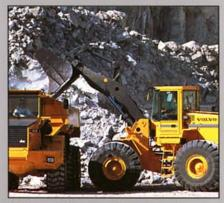
High positioned loader arms give the L180 a long reach and high lift capability which facilitates loading of high and wide vehicles.
