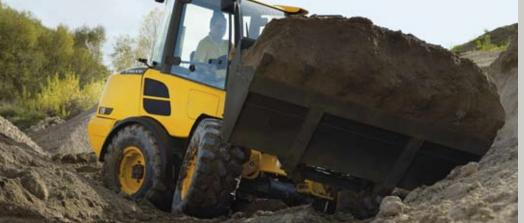
The articulating/oscillating joint keeps it stable.
