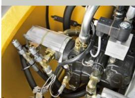
Separate working and steering hydraulic pumps.
