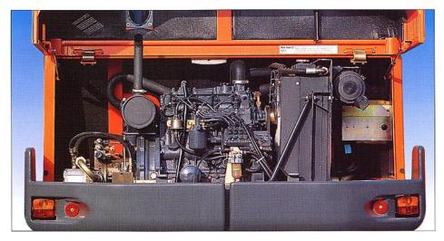
The back cover opens completely, giving excellent access to the engine and hydraulic pumps. All maintenance and checking points are conveniently located close to hand.
