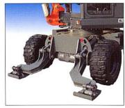
The EB 506 is equipped as standard with a sturdy blade controlled by two rams fitted with safety valves. In option, this can be replaced by two separately controlled stabilisers to which a removable blade can be added.
