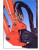
The sturdy boom king post provides a total range of movement of 130°. The double-fork pivot and the long king pin contribute to the assembly's rigidity. All the pins are fitted with bushes to ensure long life and to increase service intervals.
