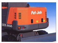
The wrap-around shape of the counterweight protects the back of the machine perfectly and makes it possible to work on the narrowest sites.
