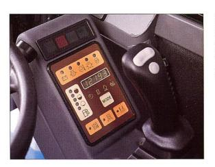
The PUMA system on the EB 506 continuously monitors all the machine's vital functions and immediately informs the operator if there is a fault. The operator is therefore free to concentrate fully on operating the machine.
