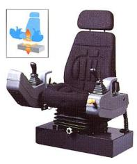
The side consoles supporting the manipulators are rigidly linked to the seat's suspension: operating precision is independent of the machine's movements and the operator is sure of finding an operating position ideally suited to him.
