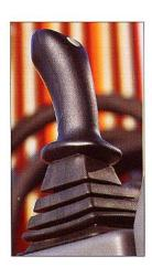
Pel-Job's new ergonomic manipulators feel good and are complemented by side arm rests which give a natural and very comfortable operating position.
