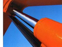
Pel-Job quality down to the last detail: the hydraulic pipes are zinc-coated and passivated for better protection against corrosion and are mounted on the top part of the boom protected from knocks. The boom cylinder's rod is fully protected against any knocks by sturdy guard. Each cylinder is well-dimensioned and equipped with cushions to absorb schock and prerent spillage.
