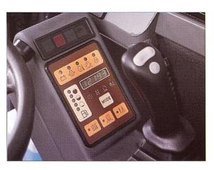
The PUMA system on the EB 706 continuously monitors all the machine's vital functions and immediately informs the operator if there is a fault. The operator is therefore free to concentrate fully on operating the machine.
