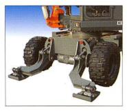
The EB 706 is equipped as standard with a sturdy blade controlled by two rams fitted with safety valves. In option, this can be replaced by two separately controlled stabilisers to which a removable blade can be added.
