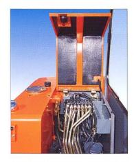
A wide central cover gives excellent access to a service platform where all the machine's hydraulic components are grouped together. Access to the control valves, rotating joint and slewing motor is immediate, which greatly facilitates all maintenance operations.
