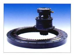
A Pel-Job exclusive: the radial piston slow slewing motor. This motor has a very high starting torque for flexible manoeuvres, and drives the crown directly without a mechanical reducer. The result is fewer moving parts and therefore less risk of wear. The automatic hydraulic brake integrated in the slewing motor immobilises the turret in all positions and guarantees optimum working safety even on a slope.
