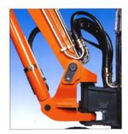
The sturdy boom king post provides a total range of movement of 130°. The double-fork pivot and the long king pin contribute to the assembly's rigidity. All the pins are fitted with bushes to ensure long life and to increase service intervals.
