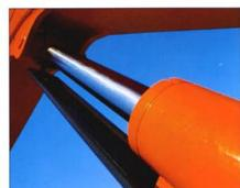
Pel-Job quality down to the last detail: the hydraulic pipes are zinc-coated and passivated for better protection against corrosion and are mounted on the top part of the boom protected from knocks. The boom cylinder's rod is fully protected against any knocks by sturdy guard. Each cylinder is well-dimensioned and equipped with cushions to absorb schock and prerent spillage.
