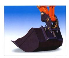
A Pel-Job exclusive: the quick coupling system available as an option enables bucket or accessory to be changed without the operator leaving the cab. Appreciated by all users, this device saves a lot of time and increases comfort considerably without altering the bucket's performances or sequence of operations.
