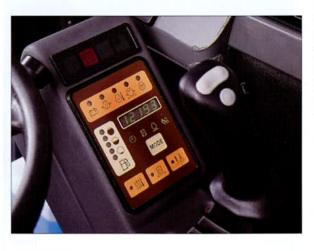
The PUMA system on the EB 706 continuously monitors all the machine's vital functions and immediately informs the operator if there is a fault. The operator is therefore free to concentrate fully on operating the machine.
