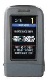
**Monitor.** The monitor is a full color Liquid Crystal Display that gives you vital operating and performance information, alerts in text, all in a simple, east to navigate format.
