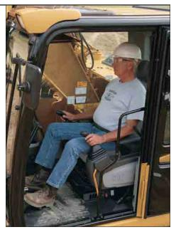
**Comfort.** The cab of the 320D LRR is the same full-sized cab with all the amenities and attachments found on the cab of the 320D L.
