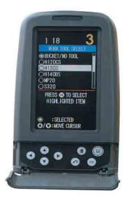
**Auxiliary Hydraulic Options.** Allows you to configure your 320D LRR to meet your work tools needs, while increasing its versatility.
