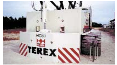
Hydraulic removable counterweight system
