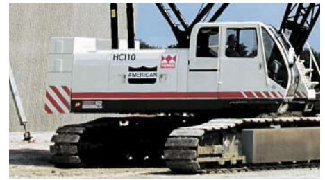
Hydraulic removable counterweight system
