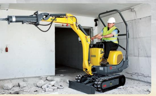
One-way hydraulics are a standard feature. Ideal for operating the specially matched Wacker Neuson hammer.
