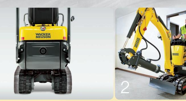
The 700 mm width of the chassis enables it to pass easily through any door, while the extended hydraulic telescopic chassis with an 860 mm external width gives it stability. It can be retracted to a width of 700 mm in no time.
