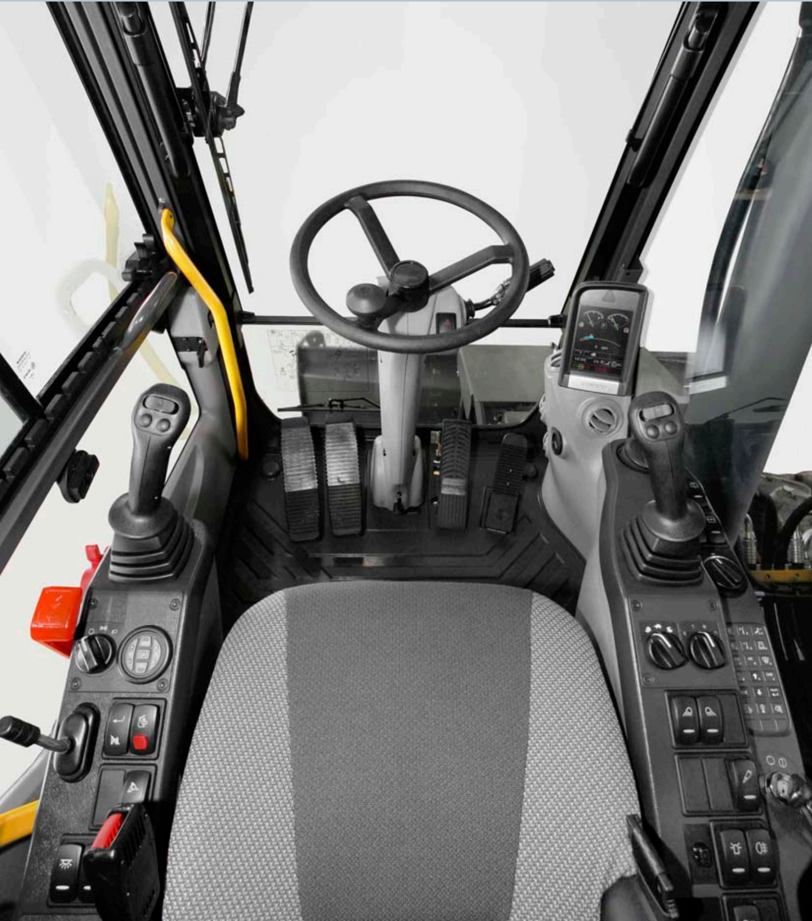
• Steering column pivots for visibility and comfort.
