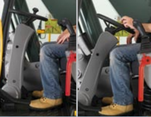
• Steering column pivots for visibility and comfort.
