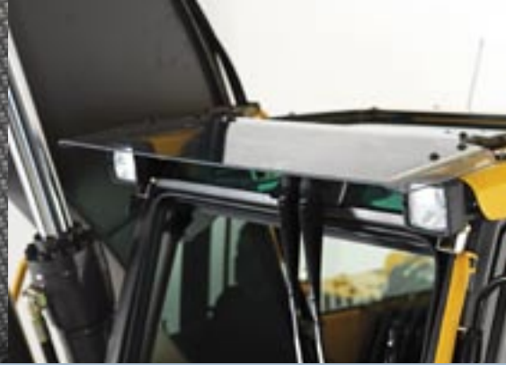
• Overhead visibility through transparent roof.
