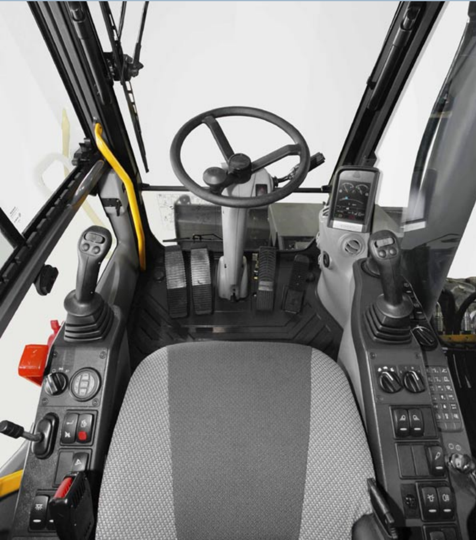
• Steering column pivots for visibility and comfort.
