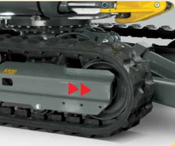
The self-cleaning crawler gets rid of dirt as it moves along.
