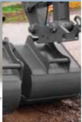
• Dedicated quick fit (left) has tightest fit, while the universal quick fit works with many bucket brands.
