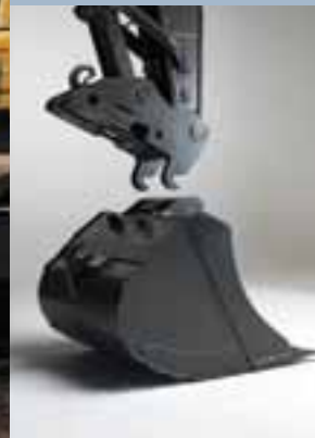
• Dedicated quick fit (left) has tightest fit, while the universal quick fit works with many bucket brands.
