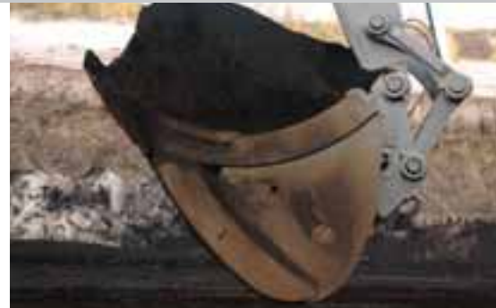
• General purpose (GP) buckets have a rugged design and self-sharpening GPE teeth.
