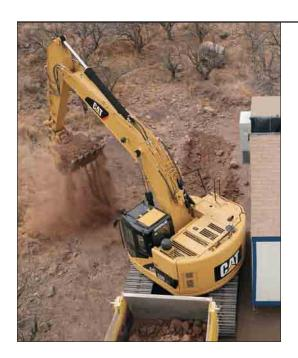
**Space Restriction.** The increasing need to work within space-restricted areas has created a demand for larger excavators that can also work within tighter quarters and provide greater productivity. The newest addition to this lineup of Compact Radius (CR) excavators is the 328D LCR.
