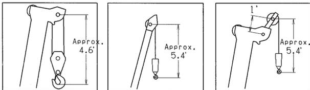
NOTE: Boom and jib geometry shown are for unloaded condition and machine standing level on firm supporting surface. Boom deflection and subsequent radius and boom angle change must be accounted for when applying load to hook.
