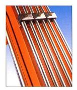
Very effective corrosion protection: all the nuts and bolts, the pins and the hydraulic pipes are zinc-plated and passivated.
