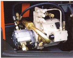
Continuous and immediate load sensing control of the hydraulic pump's flow and pressure to suit the work done by the excavator.
