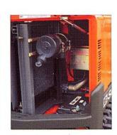
The radiators of the hydraulic circuit and engine are placed side by side to facilitate their cleaning. The battery and the air filter too are very easily accessible.
