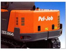
Because some knocks are unfortunately unavoidable, the wrap-around counterweight protects the rear of the machine. The steel cover is mounted recessed in relation to the counterweight to improve its protection.
