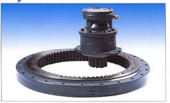
A Pel-Job exclusive: the radial piston slow slewing motor. This motor has a very high torque for flexible manoeuvres, and drives the crown directly without a mechanical reducer. The result is fewer moving parts and therefore less risk of wear. The automatic hydraulic brake integrated in the slewing motor immobilises the turret in all positions and guarantees optimum working safety even on a slope.
