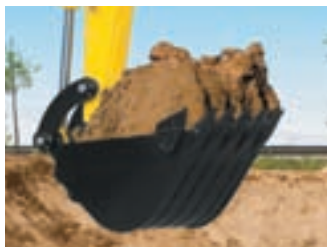
Reinforced Bucket Higher bucket link durability and anti-wear characteristics with additional reinforcement plates on cutting edge section. The bucket is reinforced with thicker steel and additional lateral plate.
