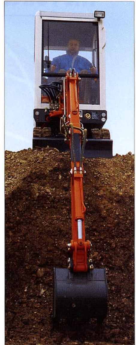
The telescopic arm available as an option increases the machine's versatility.
