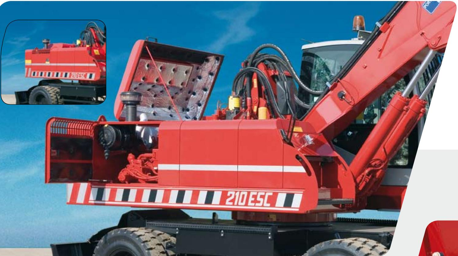
**The engine cover:** Easy access to the engine and components simplifies servicing. Internal special soundproofing covers made of polyurethane foam with a very thin sheet of lead that retains noise. Slots for air exchange turned on the top so to avoid air and noise directly on the operator.
