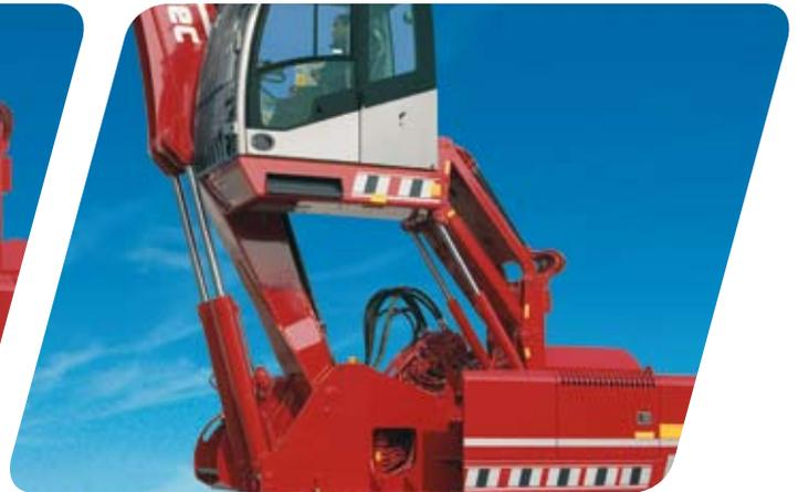
**Operators cabin** with big windows for a better visibility. The front window, with double wiper, opens, completely disappearing under the top of the cab. A rotating orange light, standard fitted, on the top of the cab guarantee a good visibility also during the darker hours of the day. It is possible, as option, to fit extra working lights on stick and on the undercarriage to increase visibility. As option it is possible to fit a front window screen or a total protection of the cab.
