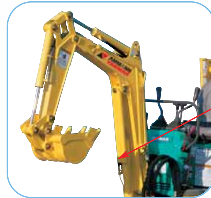
Cylinder protection on boom
