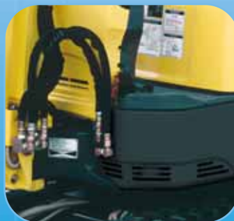
Careful routing of hydraulic pipes and hoses
