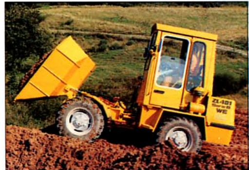
Dumper unit, 1.2 m 3 capacity
