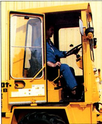
Flexibly mounted ROPS safety cab with good all-round visibility. Easy to enter and leave from both sides.
