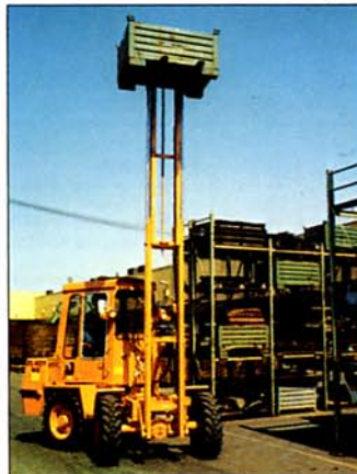
Fork-lift mast 1.5 t payload with 3.25 m lifting height* 0.6 t payload with 5.05 m lifting height*
