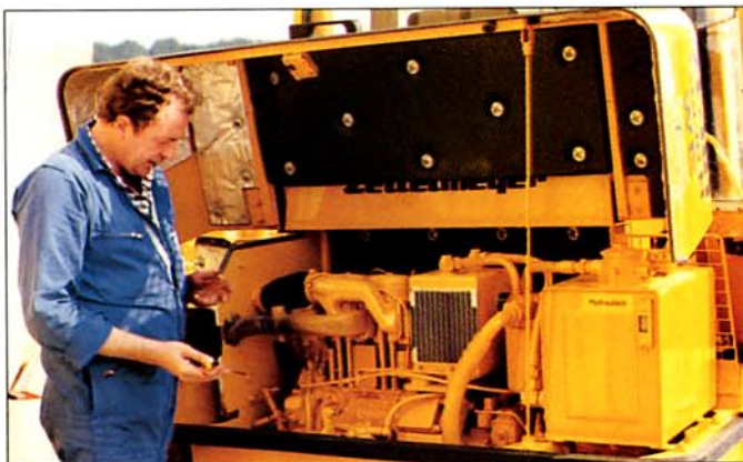
Powerful, air-cooled diesel engine – with easy access for maintenance.
