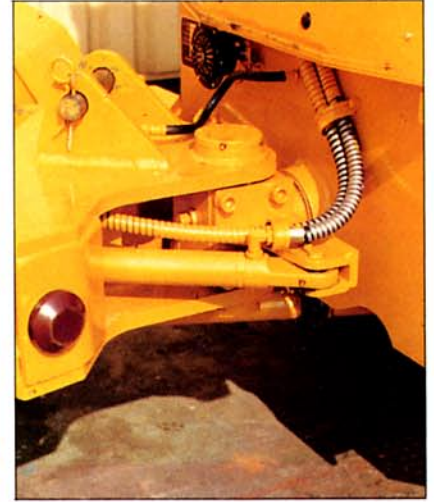
For coping with extreme operating conditions – a low maintenance articulating oscillating joint.
