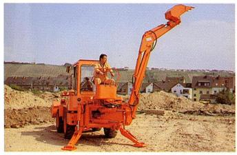
ldeal for any kind of work: extreme reach and dump height. The operator can slide the backhoe sideways by up to 1.10 m (3'7") without leaving his seat.
