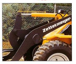
Z-bar loader-linkage - robust multipurpose loader-linkage with high breakout and lift forces. Powerful in loading and production.
