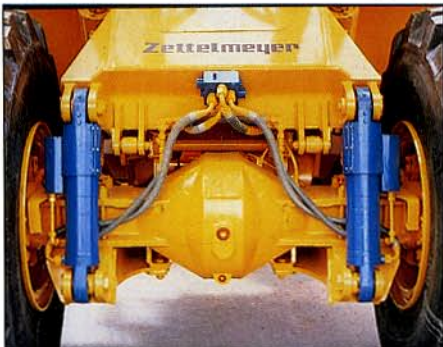
Front suspension cylinders with stabilizing valve
