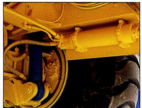
Rear suspension cylinder and accumulator
